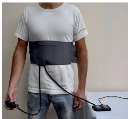
Fig. 4. Applying the belt for recording the measurement data of the respiratory rate
